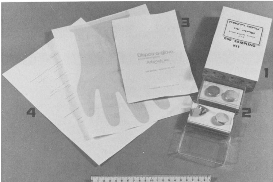
FIG. 1—Prototype field kit. 1. Cardboard box. 2. Stubs. 3. Disposable gloves. 4. Instructions and form.
